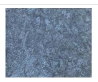
a). As polished/unetched surface showing less than 0.5% porosity
